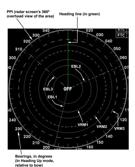
VRMs and EBLs allow you to track the distance and bearing of multiple radar targets.
